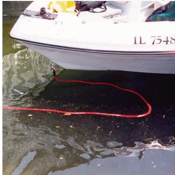
The specific gravity of polypropylene rope is less than water so it naturally floats. You won't lose a line overboard or get it caught in your propeller.
